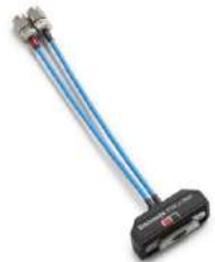
P76CA-292C 33 GHz Bandwidth Coaxial Adapter with 2.92 mm (Male) connectors and 6" of high performance cable. This adapter is calibrated at the input connectors and is ideal for directly connecting to devices with 2.92 mm or SMA output connectors.
