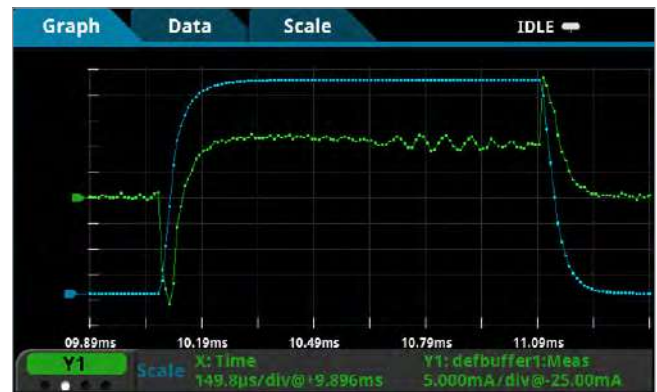
The high speed digitizing function allows capturing and displaying voltage and current measurements simultaneously.
