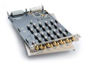
The 3761 provides quality low-current switching at an affordable price. The offset current error generated is specified <1 pA, with typical performance at <30 fA. When used with a voltage source and an electrometer or picoammeter, this card can easily automate insulation resistance tests, reverse leakage tests on semiconductor junctions, or gate leakage tests on FETs.
