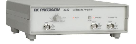
The 3030 is a DC to 1MHz amplifier with a maximum output of 30 volts peak to peak from a 50  $\Omega$  source impedance. A 600  $\Omega$  output is also provided. The unit can output up to 15 volts peak to peak into a 50  $\Omega$  load and can drive up to 300 mA peak into a low impedance or short circuit.
