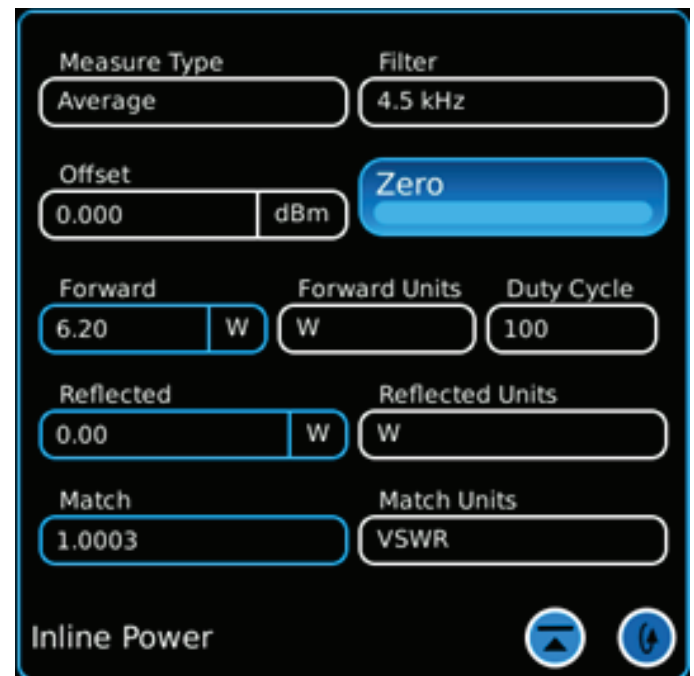
In-Line Power Meter Tile
