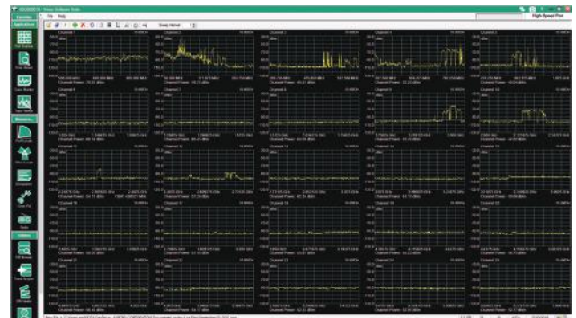
Use the High Speed Port Scanner Monitor Multiple RF Channels with a Single MS2090A on a Single PC Monitor
