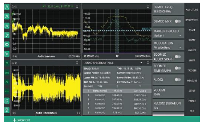
The AM/FM Modulation Measurements Screen Provides a Unique Simultaneous Display of Results and RF and Audio Spectrum
