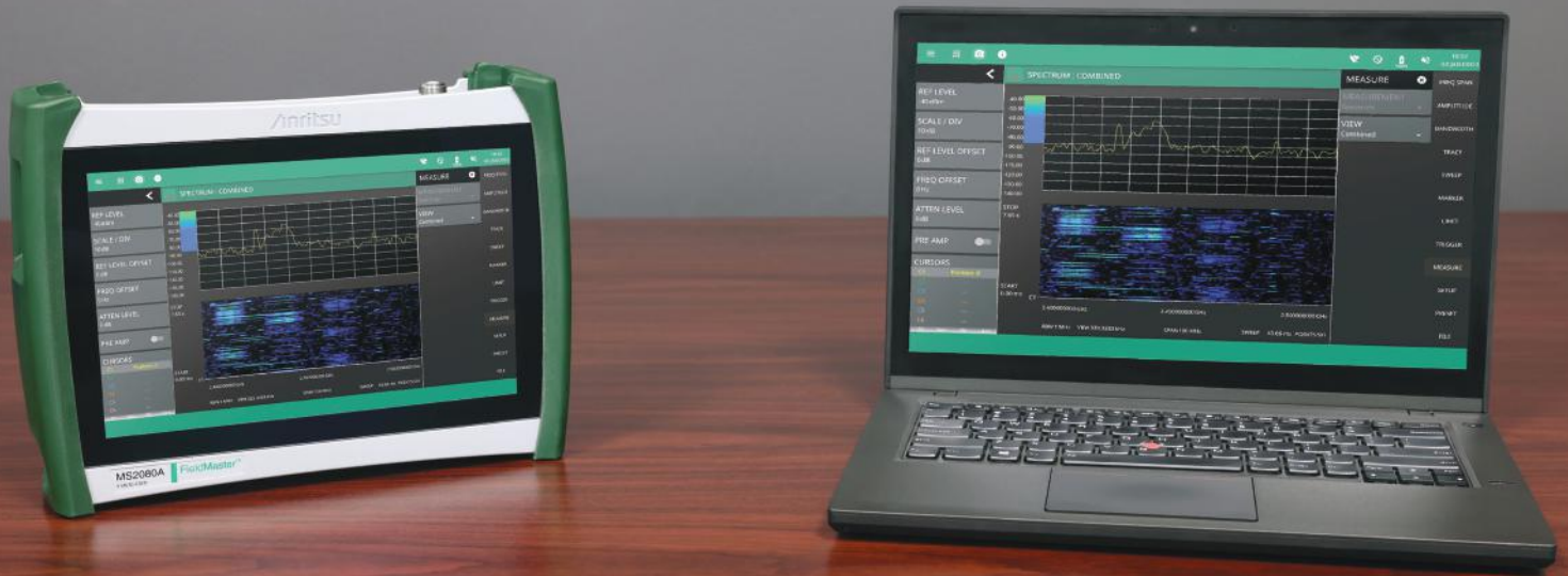
Laptop PC Running Remote GUI Application with Wi-Fi Connection to MS2080A
