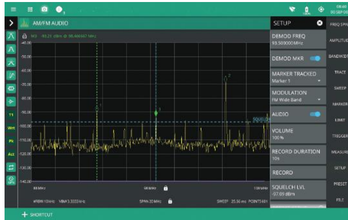
AM/FM Signal Demodulation at Marker Frequency
