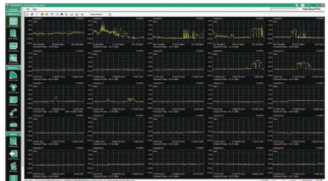
Use the High Speed Port Scanner Monitor Multiple RF Channels with a Single MS2080A on a Single PC Monitor
