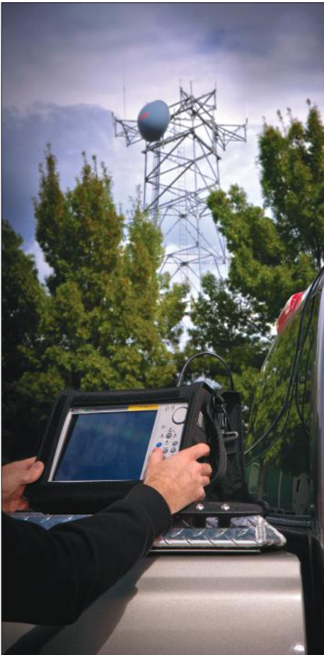
LMR Master testing from a service vehicle
