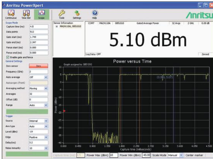
Measurement of average power in slot 4 of TD-SCDMA waveform via time gating feature of MA24118A using PowerXpert.
