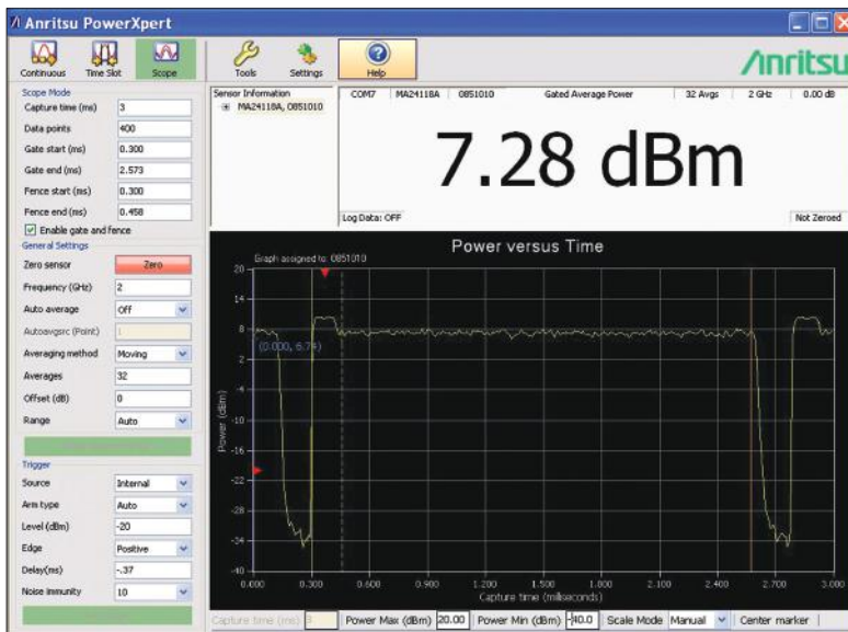
Measurement of average power of a WIMAX burst while excluding the effects of preamble via gate and fence feature of MA24118A using PowerXpert.
