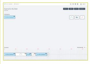
The realism of the network experience can be further enhanced by adding intelligent transitions between each element. Transitions define how NE-ONE Professional will handle the changes, for example a variable transition from a 4G to 5G network or perhaps a momentary outage between the change.
