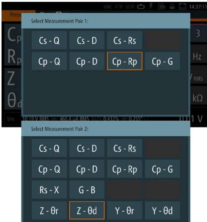
Measurement functions can be selected in pairs
