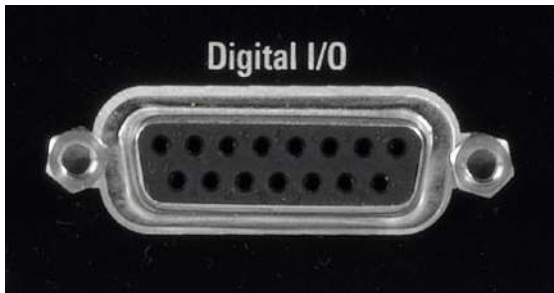
Digital I/O ports on rear panel
