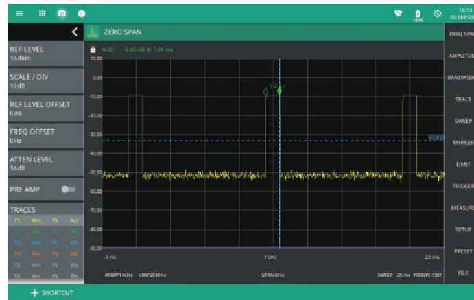
Use Zero Span to View Radar Pulses and TDD Transmitters
