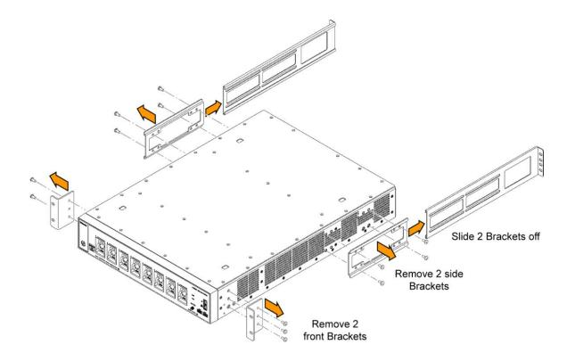
**3.** Remove the three screws from the rack mounting bracket at the right-front of the instrument and remove the bracket.
