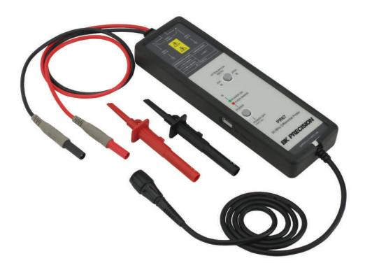
Differential probes enable earth grounded oscilloscopes to make safe and accurate floating measurements between two voltage points. The PR65 Series differential probes convert floating signals to low-voltage ground-referenced signals that can be displayed safely on any ground-referenced oscilloscope.
