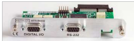
KTTI-RS232 RS-232 interface with 6 digital I/O ports.
