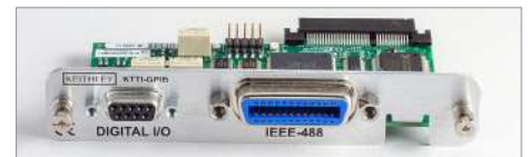
KTTI-GPIB GPIB interface with 6 digital I/O ports.
