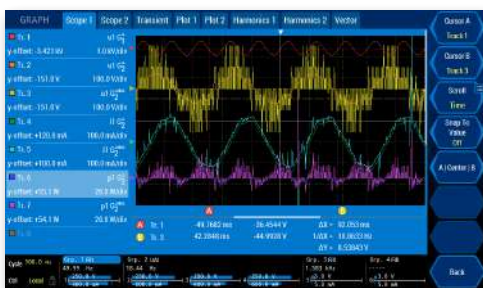
Simultaneous measurement of narrowband and wideband values
