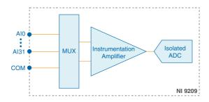
Input signals are scanned, buffered, conditioned, and then sampled by a single ADC.
