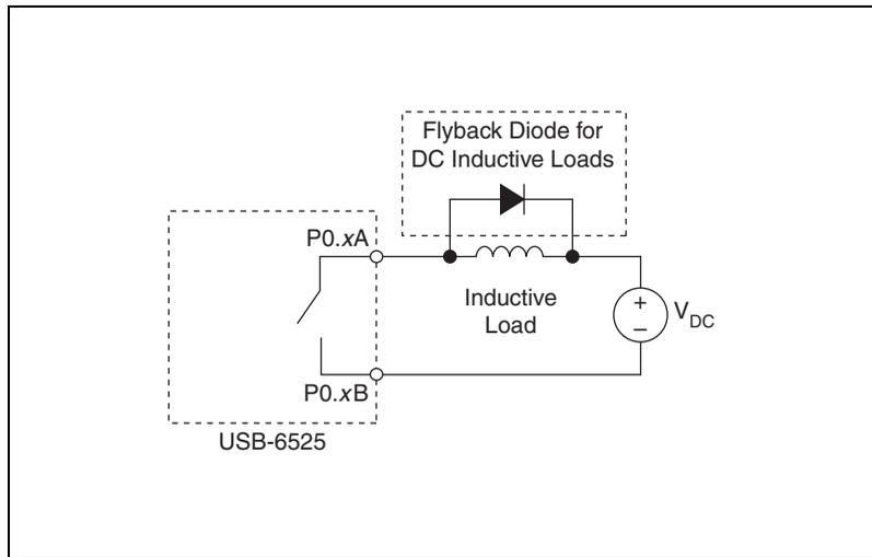
**Figure 8.** Contact Protection for DC Inductive Loads
