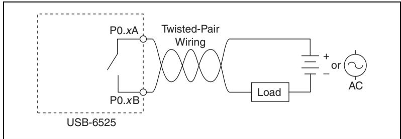
**Figure 7.** Connecting a Load to the USB-6525
