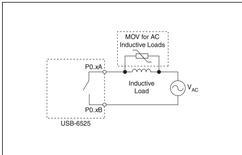
**Figure 9.** Contact Protection for AC Inductive Loads
