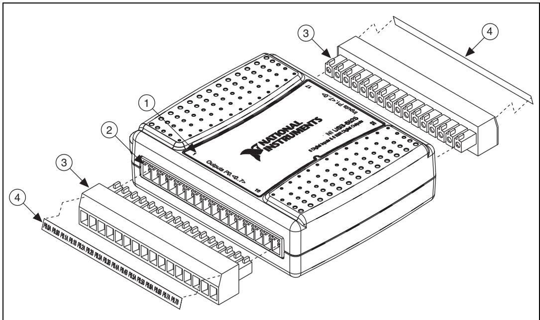
1 Overlay Label with Pin Orientation Guides
