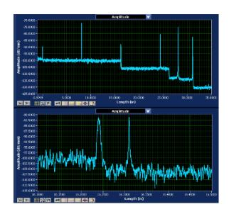
**Top**: OBR 4200 measurement of an optical fiber harness with a bend loss and splice loss **Bottom**: Easily distinguishable bend loss 7 cm before a connection
