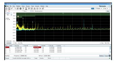
Analysis of AM and FM signals is standard in SignalVu-PC. The following screen shot shows a 1 kHz tone amplitude modulating a carrier to 48.9% total AM. Markers are used on the spectrum display to measure the modulation sideband at 1 kHz offset, 12.28 dB down from
