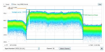
In this illustration, a single region has been selected. Since we have declared this to be an ATSC video signal, the spectrum mask for the ATSC signal is shown overlaid in the region. The signal is a close match to the spectrum mask, including the vestigial carrier at the lower side of the signal, characteristic of ATSC broadcasts.
