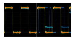
R&S®RT06 oscilloscopes can update at a high rate of up to one million waveforms per second when histograms, masks or cursor measurements are active. The ASIC based signal processing paths ensure a smooth workflow even when performing analysis with the deep acquisition memory.
